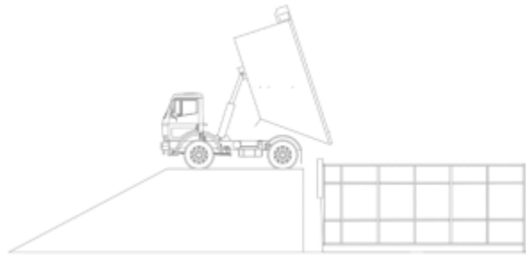
Figure 60: Transhipment operation from tank vehicle to roll-off container
