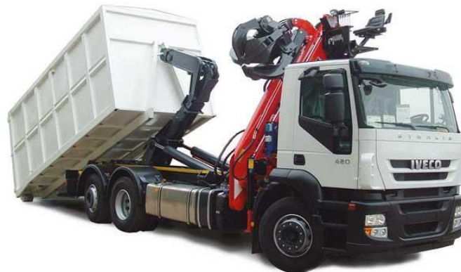
Figure 61: Open-top trailer hooking up a roll-off container
