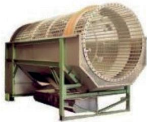
Figure 5. Drum for desalting of hides Source: www.rizzi.it
