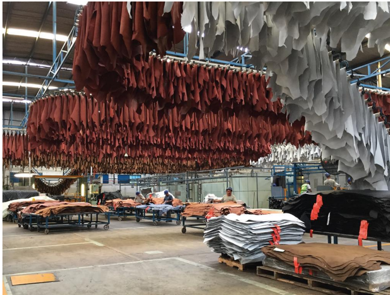
Figure 9. Overhead chain conveyor drier Source: N. Niedzwiedz
