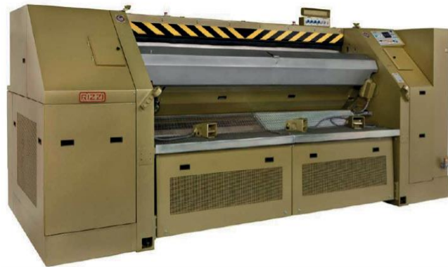
Figure 6. Through-feed fleshing machine Source: www.rizzi.it
