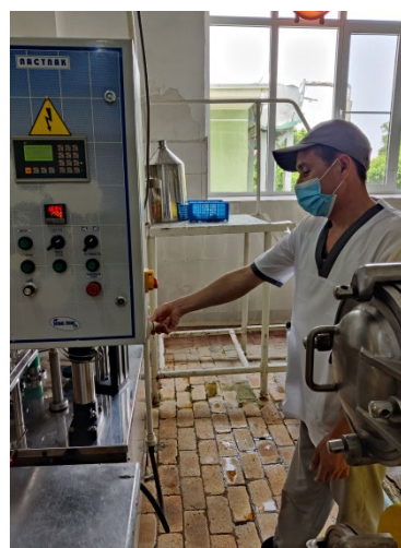
Image 4, After: Pneumatic machine after compressed air leaks were stopped
