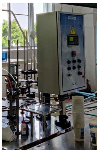
Image 3, Before: Pneumatic machine where major compressed air leaks were found
