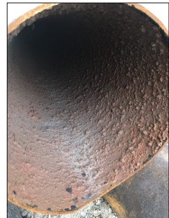
Photo 2.2 Removal of corroded pipe. Credit: COWI
