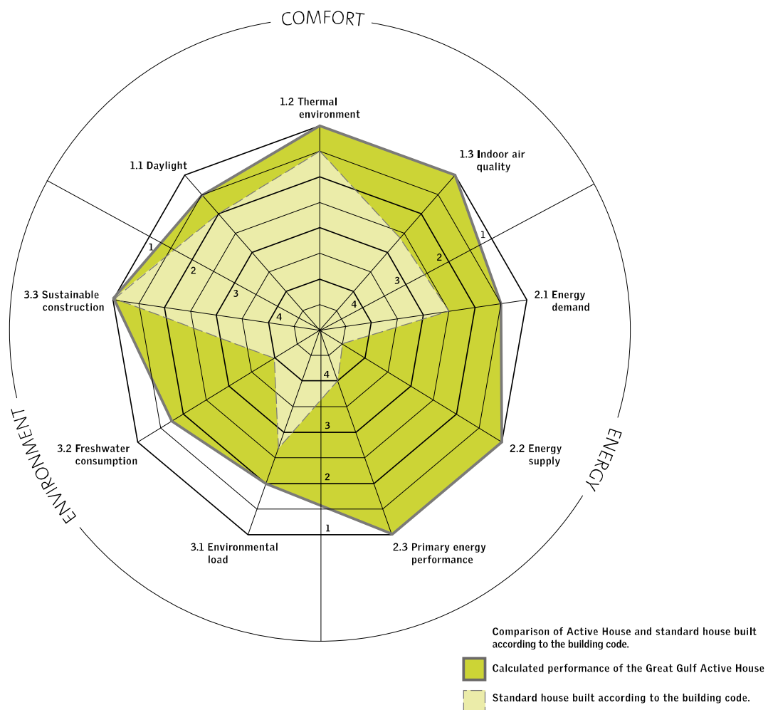
Figure 6-9 : Comparison of Active House against a house built to standard. (Source: Active House Alliance).
