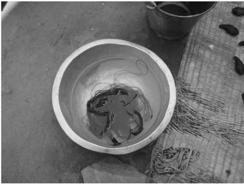
Wax wires dipped in water
