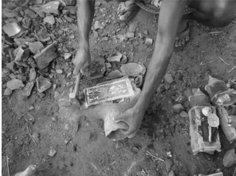
Clay mould being broken with small hammer
