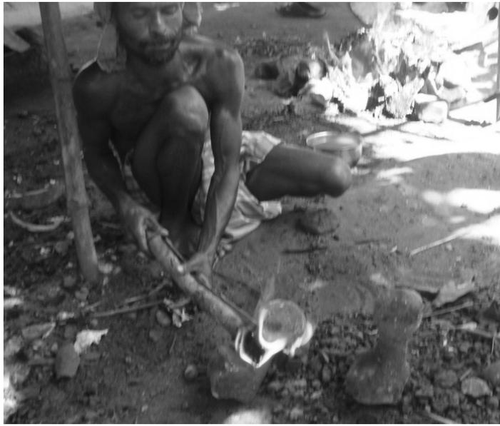
Piece being inverted using bamboo tongs
