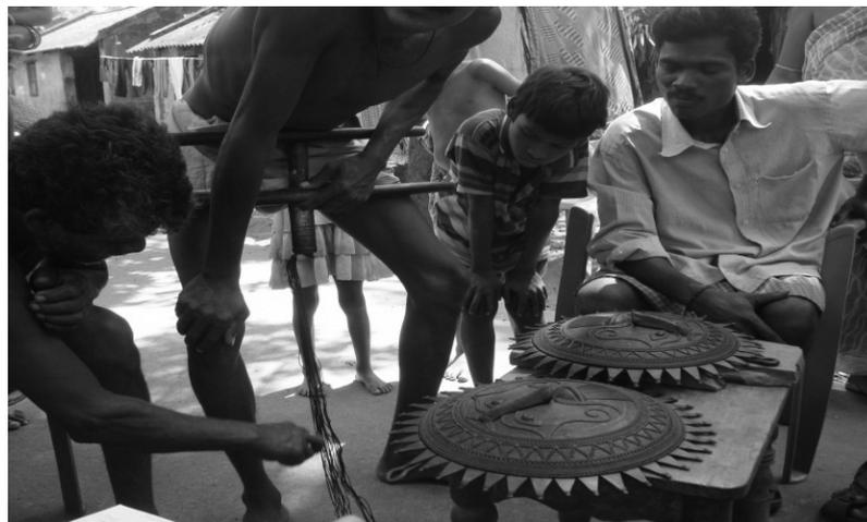
Working of the extruder to make wax wires
