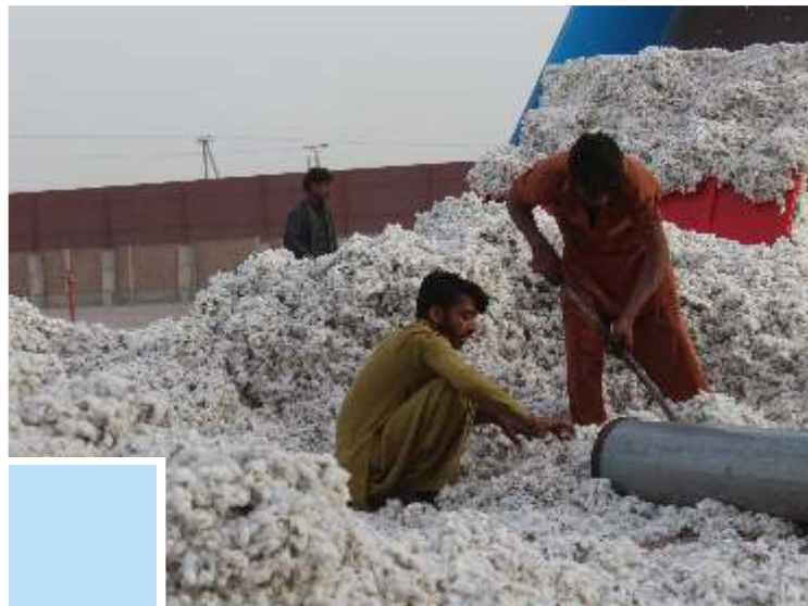
Seed Cotton feeding through suction pipe
