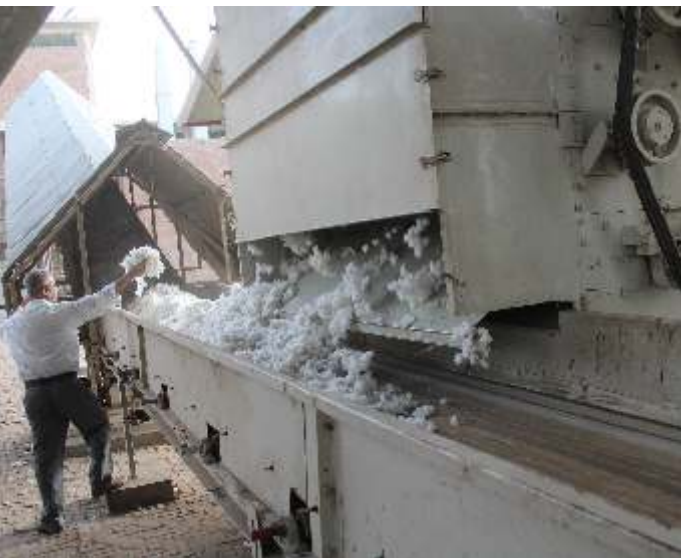
Seed Cotton transportation through conveyor belt
