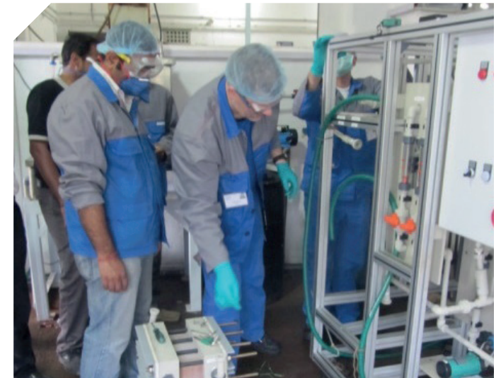
Mounting of diffusion dialysis stack in Chennai
