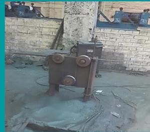
Mechanical descaling process instead of pickling process is now used for low carbon steel. This has significantly reduced the consumption of HCl to 615,673 litre only.
